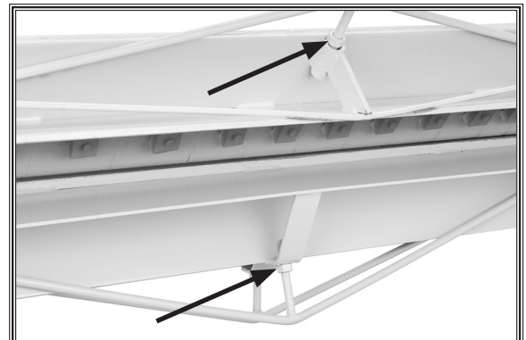
Figure 18. Bending wing mounting bolts.
